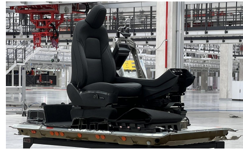
Fig. 1. Tesla 4680 structural battery pack with seats pre-attached for final assembly [8].
