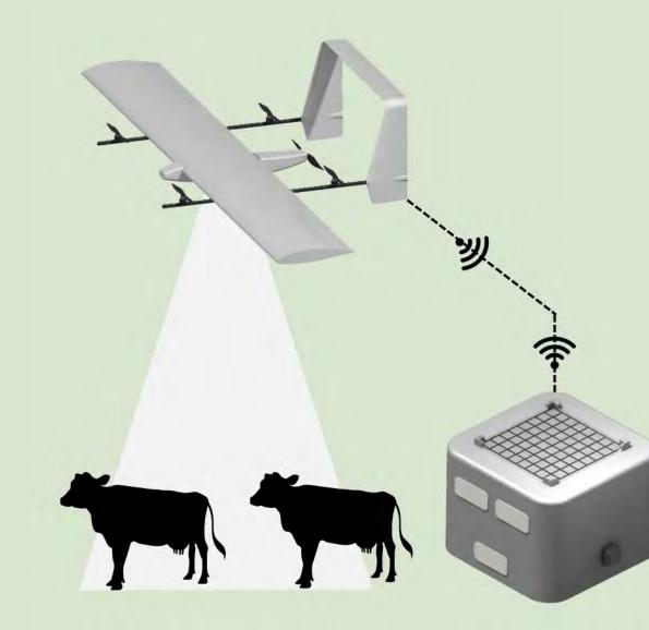
Aeroacoustically optimized cruise propellers operate with minimal interference with spectrum of frequencies cattle are sensitive to for low-stress cattle management.
