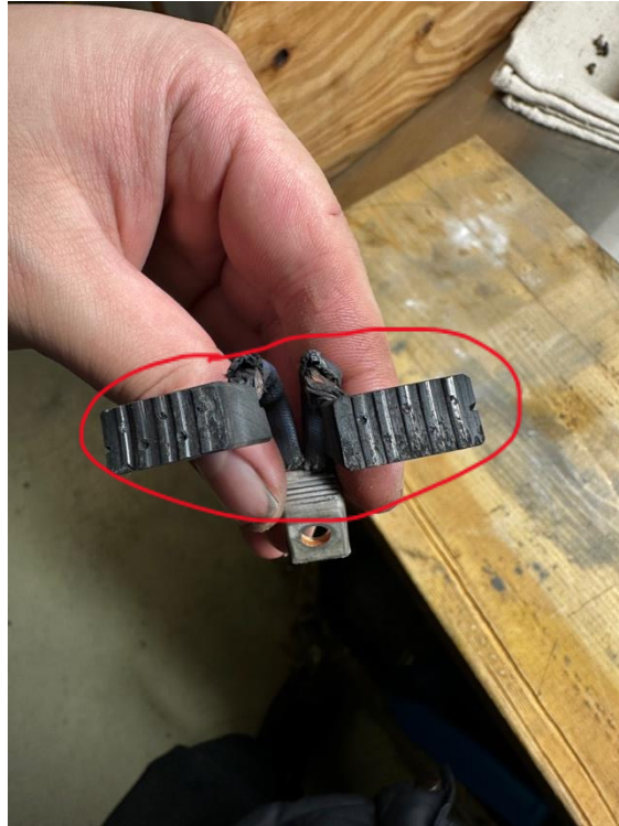
2. C-208 PT6engine -Starter Generator carbon brush abnormal wear
