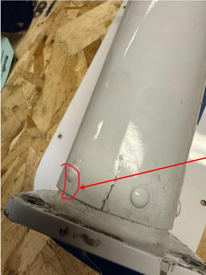
Cessna 208- Elevator Torque tube crack
