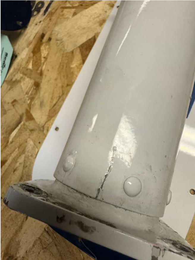
Cessna 208 – Elevator Torque tube crack
