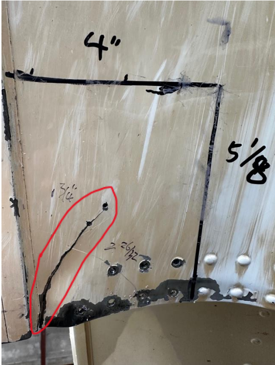
1. C208 Wipaire 8000 float overlooked Crack under float skin
