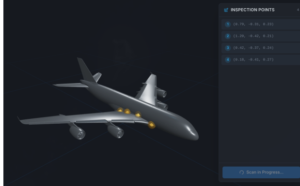
Figure 3: User interface for the digital twin and inspection data visualization.
