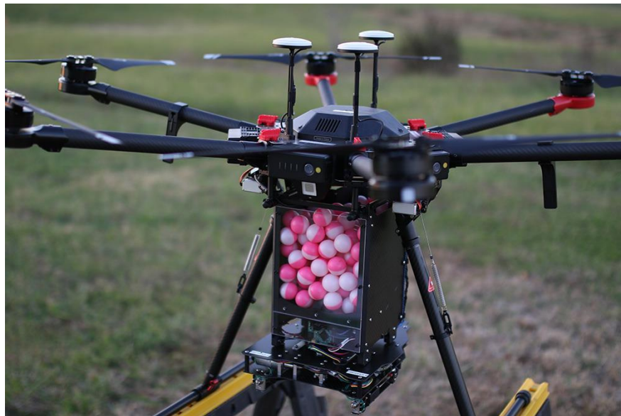
Figure 1 'Ignis' drone by Drone Amplified. "Drone Amplified's IGNIS payload system." FlyingMag, October 7, 2021, https://www.flyingmag.com/drones-wildfire-fighting/ .
