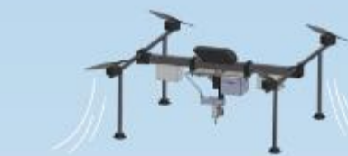
4 - Fly to coordinates. Wet soil and wait. Probe soil and store data with coordinates. Fly to next coordinates.
